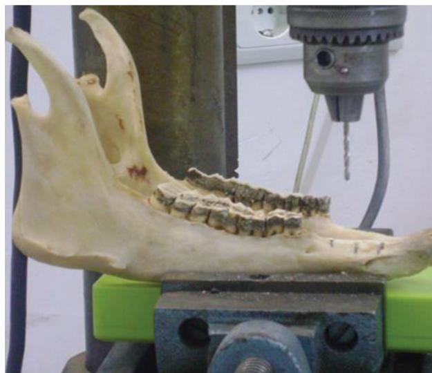
Fig. 3 Parallel drilling of implant holes.
