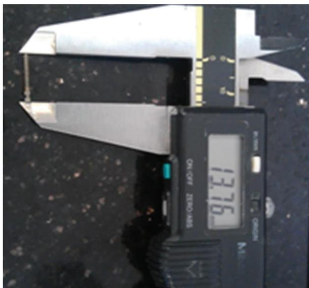
Fig. 1 Pin length measurement by digital caliper.
